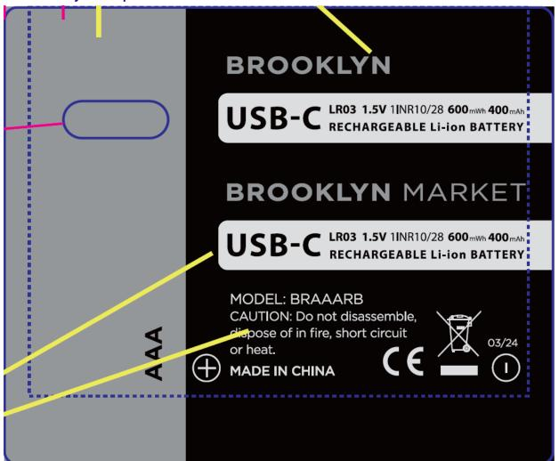
Remark: 1. Terminal of battery pack has clear polarity marking on the external surface; 2. '03/24' refers to manufacturer date, '03' refers to months, '24' refers to years.
